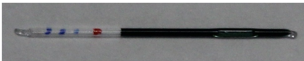
Fig. 8. Micro cell made of a quartz capillary: outer diameter of 1 mm, inner diameter of 0.5 mm and 25 mm length. Both the purification and sealing processes are performed in an ultra-pure vacuum glove box.
